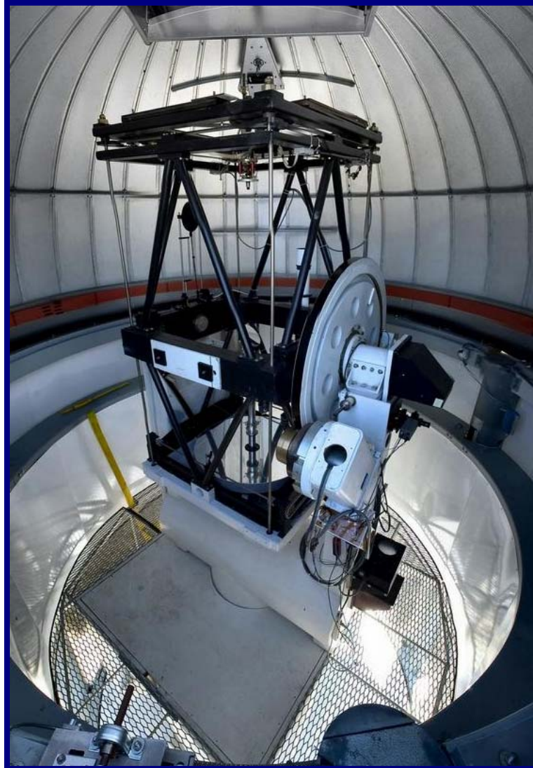
Figure 3. One of the six CHARA telescopes shown in its enclosure. The primary, secondary and tertiary mirrors can all be seen inside the main telescope tube. The large wheel on the right is the elevation drive while the azimuth drive is hidden below the floor. The M4 and M5 mirrors are contained inside the black boxes on the right of the telescope. Between these two mirrors is a large area of collimated beam used for acquisition, and will, in the future, allow the installation of an adaptive optics system.
