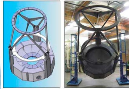
Figure 12 (Left) 3-D design of the NPOI 1.4m Cassegrain telescope (Right) Assembled NPOI Telescope shown in assembly structure at CMA. Complete OTA weight is 115 kg. The telescope is being painted and optics will be completed the end of 2007.
