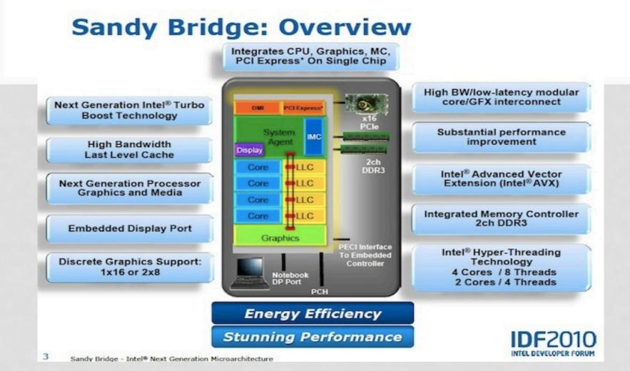
Intel updated the ring-bus controller to integrate and connect all subcores, increased performance and efficiency and lower latency.
