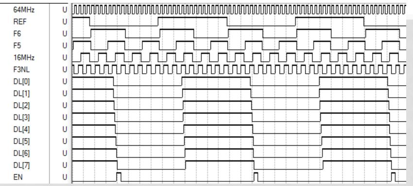
Using above generated clocks,  $\lambda$  /32 can be detected. Using the heterodyne frequency of 2MHz, this results in 15.625ns precision. Higher resolutions are achieved by latching 8-tap monolithic delay lines with 2ns tap-to-tap delay.
