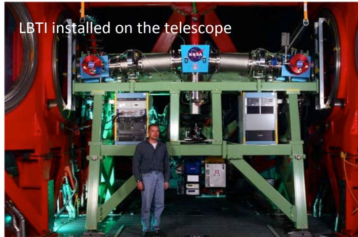
LBTI installed on the telescope
