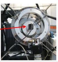
Measurements showed astigmatism which cannot be related to the optical alignment of the telescope since M2 was not involved. However, the WFS optics could still be astigmatic.
