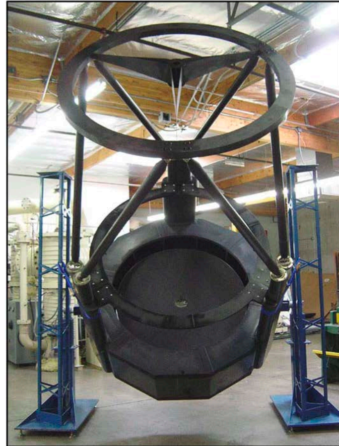
Figure 12 (Left) 3-D design of the NPOI 1.4m Cassegrain telescope (Right) Assembled NPOI Telescope shown in assembly structure at CMA. Complete OTA weight is 115 kg. The telescope is being painted and optics will be completed the end of 2007.
