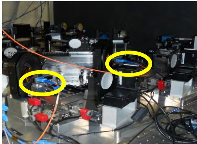
Connection of the ALOHA fibers into the FLUOR injection module
