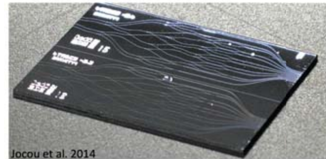
Fiber-to-GRAVITY interface made at IPAG
