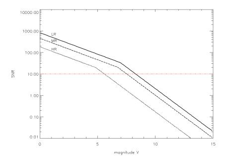
Fig. 5: SNR calculations for the three different spectral resolutions. The hypotheses on the spectral bands are the same than in figure 4. The calculations are made for a seeing of 1.25" (median conditions) and 30mn of integration time.
