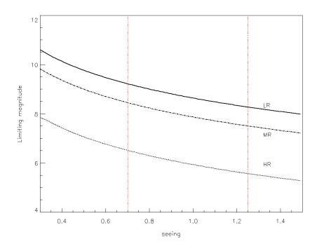
Fig. 4: Limiting magnitude for 30mn of integration, a signal to noise ratio of 10 on the differential visibility measurement with  $\Delta\lambda_1$ = 50 nm (resp. 40, 6.7) and  $\Delta\lambda_2$ = 0.4 nm (resp. 0.13, 0.02) for the Low LR (resp. medium MR, high HR) spectral resolution and a central wavelength equal to 650nm. The vertical lines correspond to the median and excellent seeing conditions.
