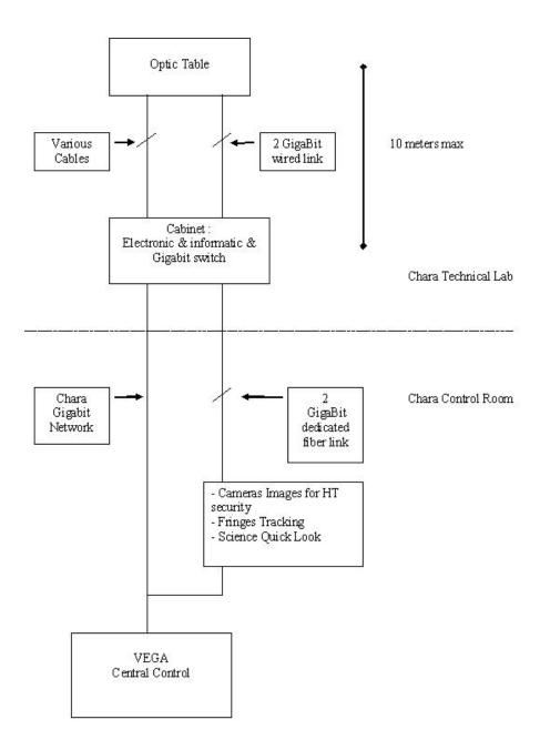
Fig. 9: Hardware implementation of the VEGA control system
