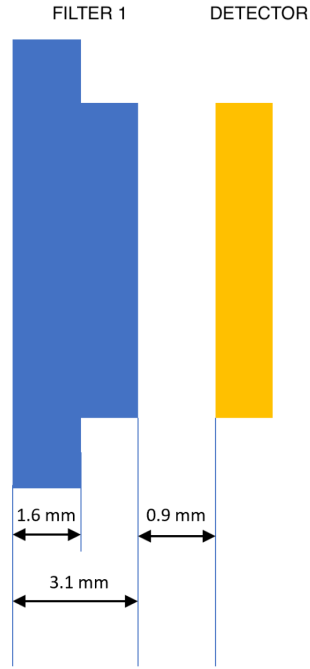
Figure 7. Proposed shape of edge filter to replace filter #1.
