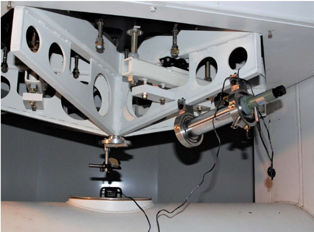
Figure 10. The setup for centering M2 mount on the telescope axis. The relay mirror is hanging from a base that extends to grab the inside of the middle tube. The custom clamps on the Brunson alignment scope were designed to grab the M1 mount.
