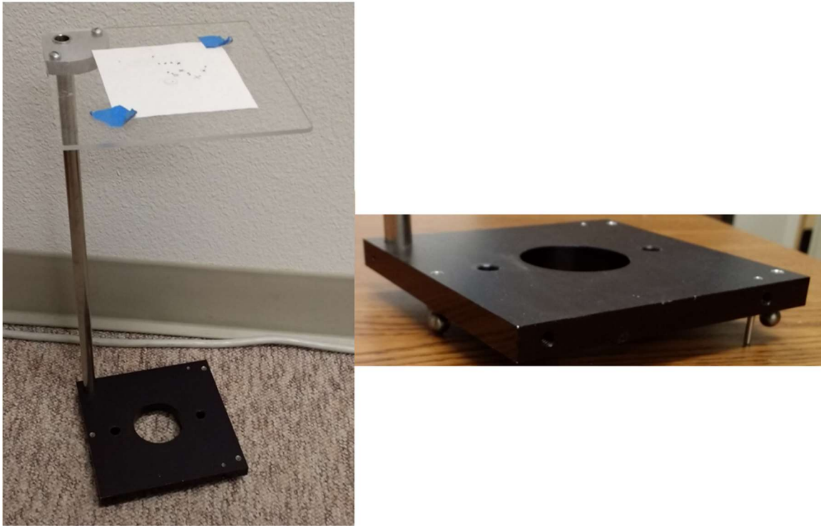
Figure 2. The alignment jig to be placed over the M6 hole. This jig is useful for checking M7 position with respect to the azimuth axis and for setting M7 tilt initially.
