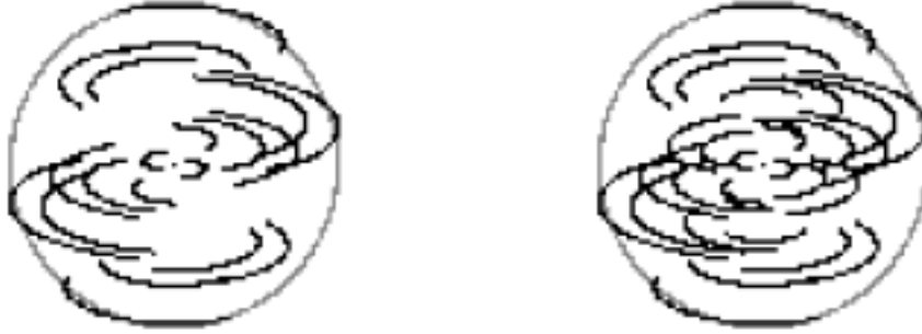
FIGURE 2. Left: UV coverage with optimum 5-telescope configuration. Right: UV coverage including 100-inch Telescope. The outer circle represents a 354m separation, as in the original CHARA Y.
