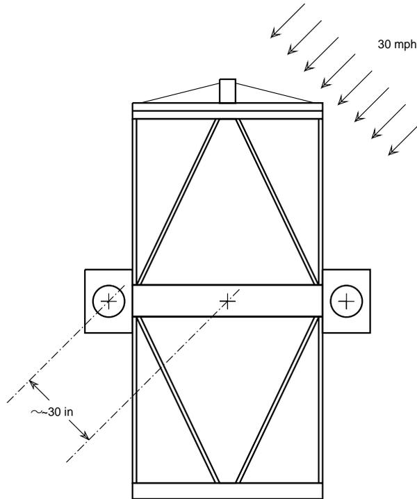
FIGURE 4. Wind torque on the azimuth drive.
