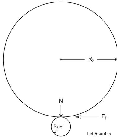
**FIGURE 5.** Friction on roller interface.
