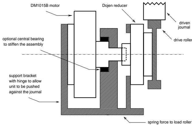
FIGURE 7. Schematic of drive unit configuration.
