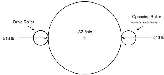
FIGURE 6. Azimuth axis with drive and opposing rollers.
