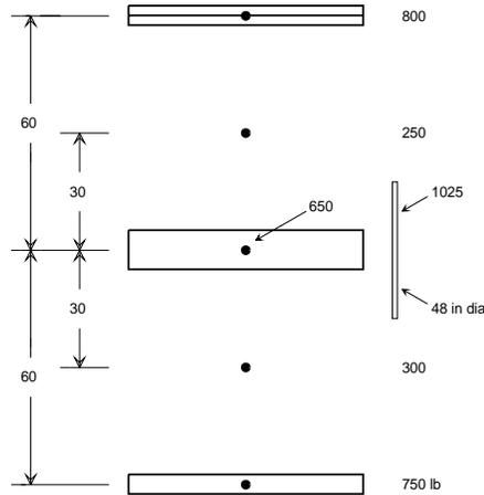
**FIGURE 3.** Weight distribution assumed for torque estimate.
