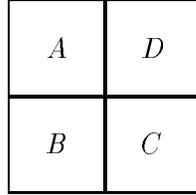
**FIGURE 2.** Definition of quadrant detector channels as viewed from the front of the quadrant detector.
