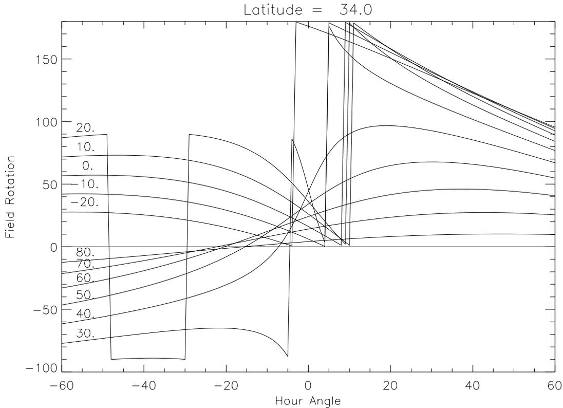
**FIGURE 3.** Rotation of telescope axes on quadrant detector for a range of declinations.
