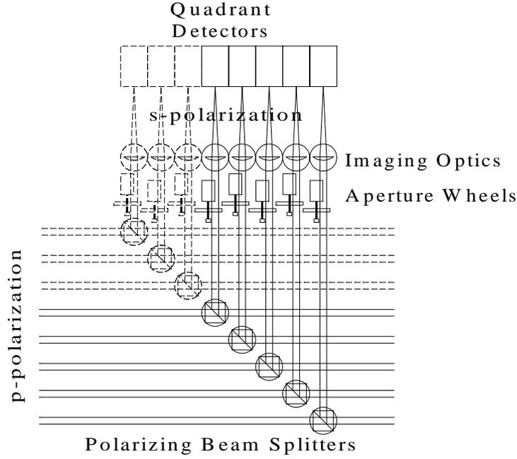
**FIGURE 1.** Schematic of the Wobbler optical layout.
