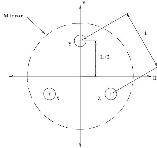
**FIGURE 4.** The axes used to define mirror response. The position of the mirror can be represented as a vertical and horizontal tilt ( $V$  and  $H$ ) or as the positions of the three actuators ( $X$ ,  $Y$  and  $Z$ ).
