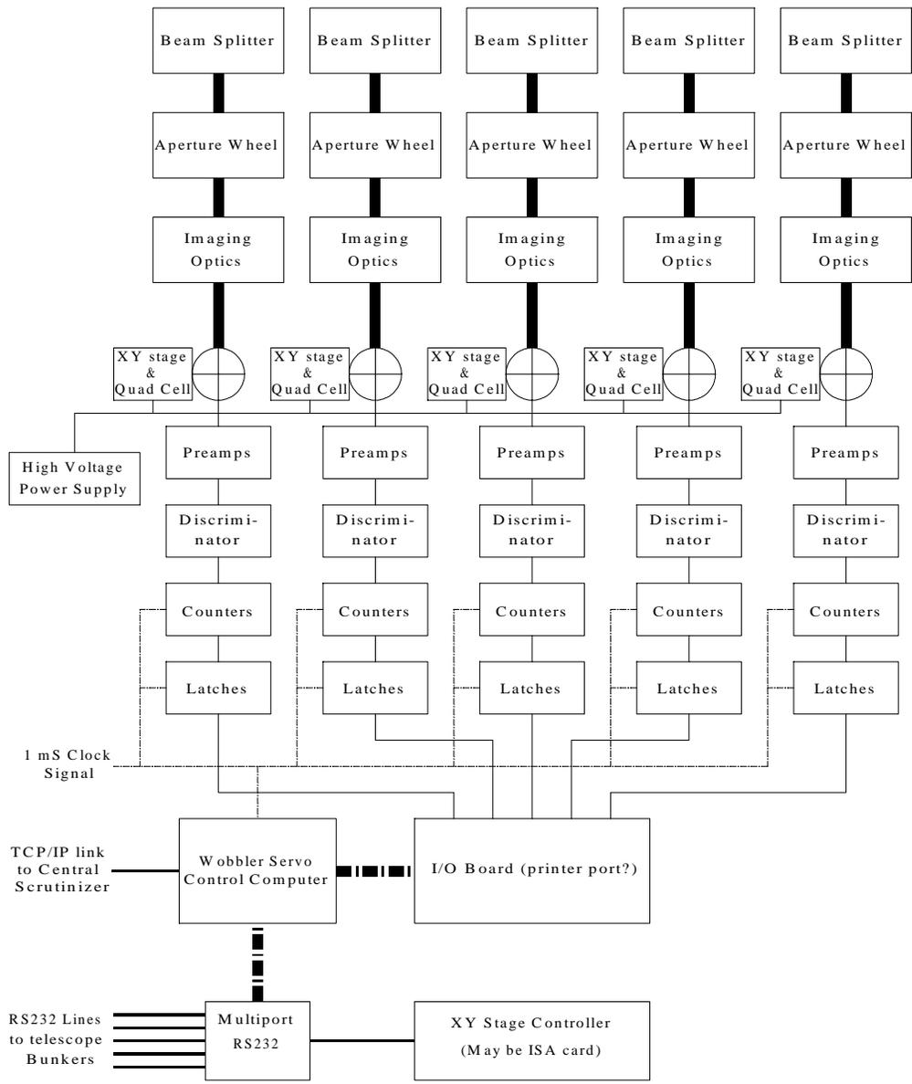
FIGURE 5. Schematic of the Wobbler servo control system hardware.
