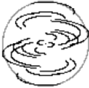
FIGURE 2. Left: UV coverage with optimum ‘3 arm’ 5-telescope configuration. Right: UV coverage with best 3+2 configuration. The outer circle represents a 354 m separation, as in the original CHARA Y.
