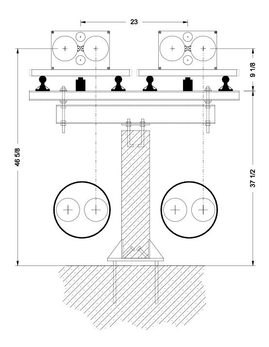
**FIGURE 1.** Nominal dimensions for the OPLE T support system as viewed from the west. The dotted lines mark the place where the light moves from the POPs in to the OPLE.
