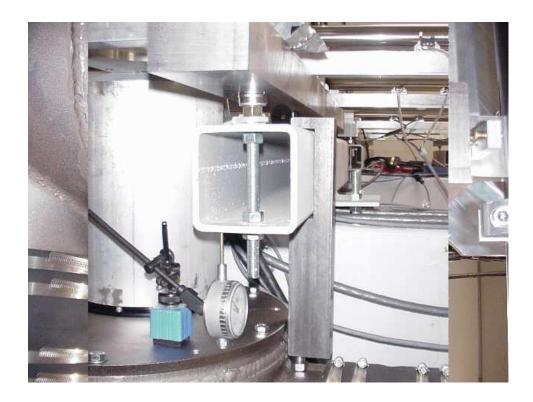
**FIGURE 5.** Image showing the steel notched brace located under the square beam. The notch fits into the beam, while tension screws above and below adjust the desired stiffness.
