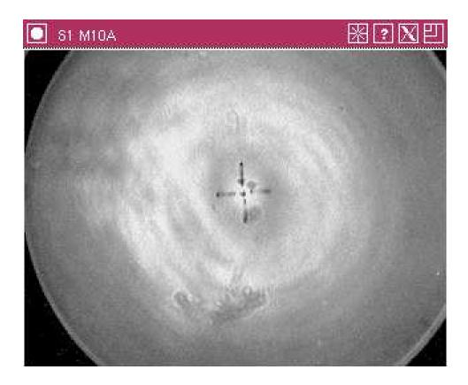
**FIGURE 1.** An example of an M10 image from the S1 telescope TV monitor, with DL cart in back position. This position serves as the (0,0) image position for S1.
