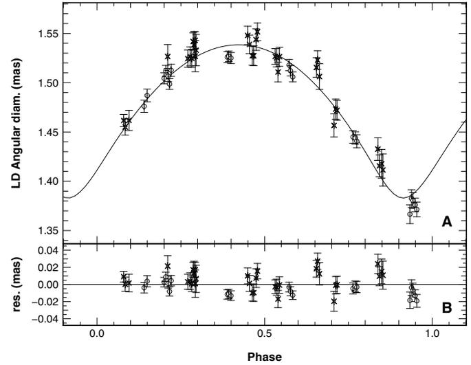
**Fig. 2.**  $p$ -factor determination. A. Our angular diameter measurements (points). Crosses correspond to the medium baseline (E2-W1), while circles correspond to the largest baseline (E1-W1). The continuous line is the integration of the 4-knots periodic cubic spline fitted to the radial velocities (Fig. 1). Integration parameters:  $\bar{\theta} = 1.475$  mas,  $p = 1.269$  and  $d = 274$  pc. B. Residuals of the fit.
