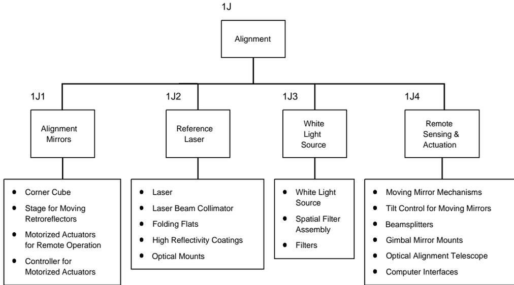
**FIGURE M.1.** Hardware tree for the alignment subsystem.
