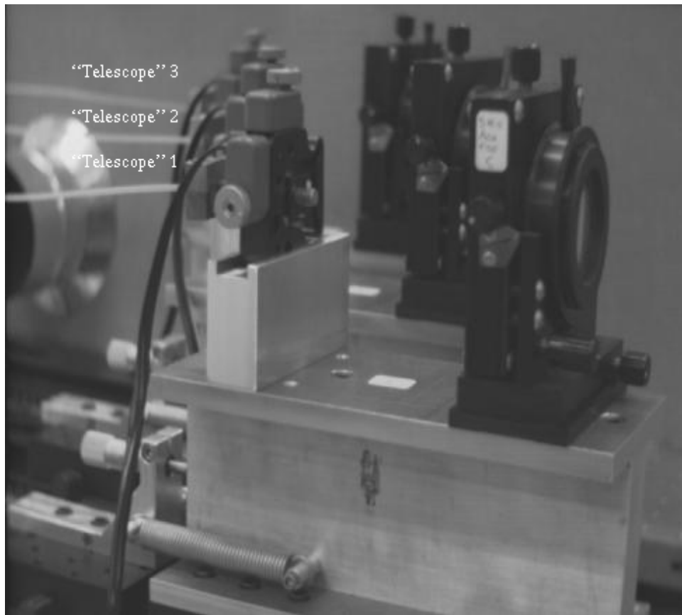
Figure 4. A view of the Fiber Launcher system from slightly above the optical axis height. Note that the three input beams are labelled as “Telescope” 3, “Telescope” 2, and “Telescope” 1.
