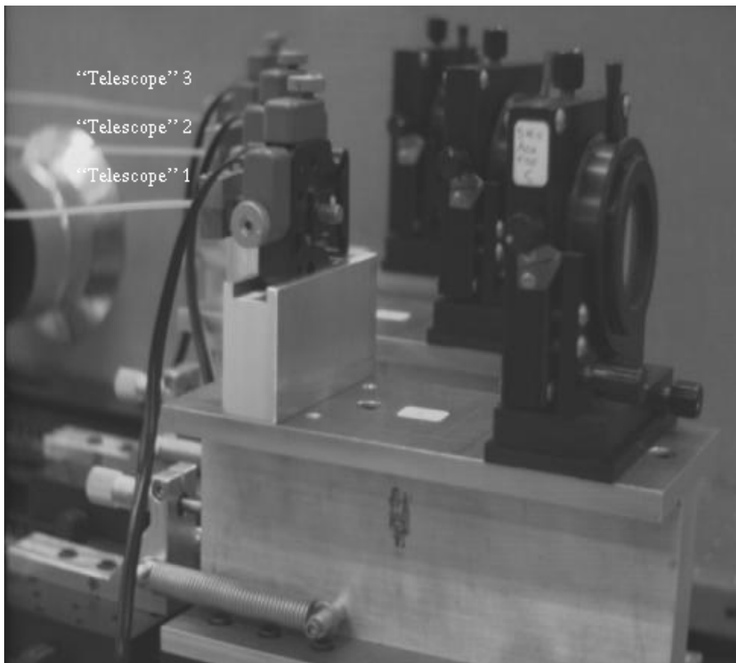
Figure 5.1: A view of the Fiber Launcher system from slightly above the optical axis height. Note that the three input beams are labelled as “Telescope” 3, “Telescope” 2, and “Telescope” 1. These labels are maintained throughout this dissertation.
