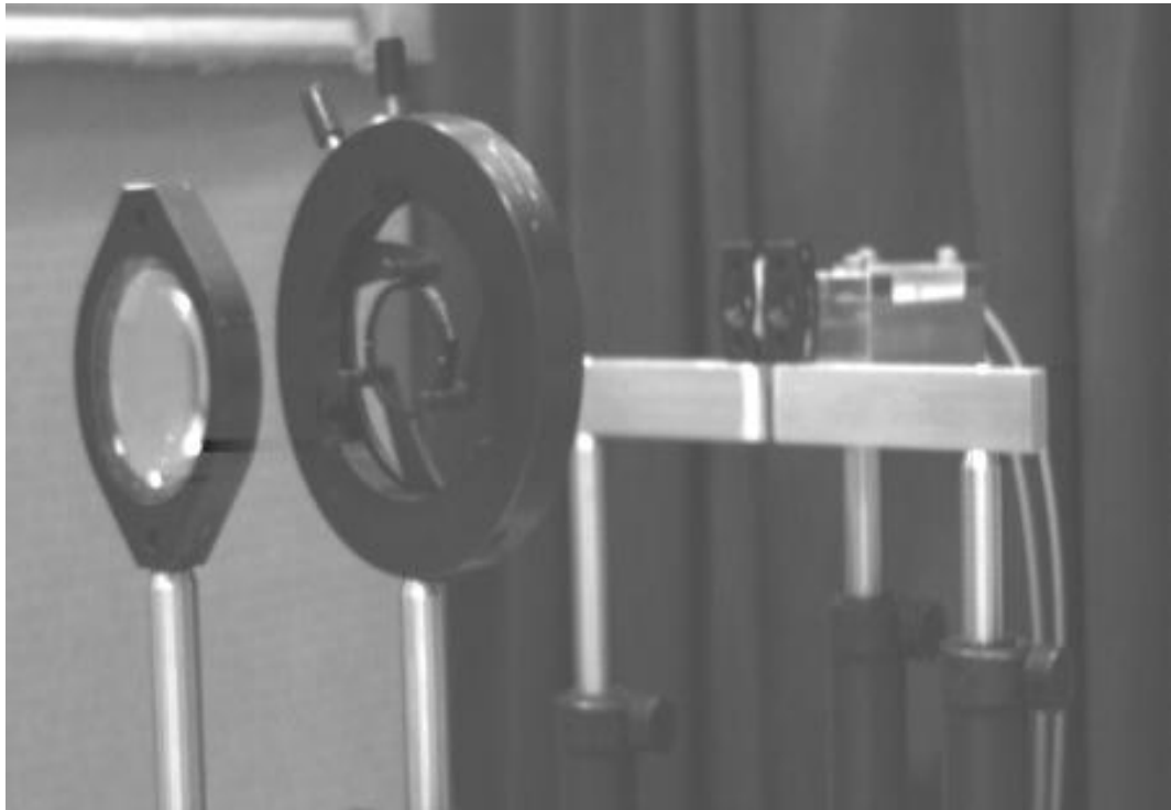
Figure 6.1: The experimental setup for acquisition of fringes with two beams. The light exits the fiber at the right of the figure, being first collimated, then sent through a polarizer, then re-imaged with the lens on the left of the figure to a microscope objective (not shown) which magnifies the image for detection by a CCD video camera (not shown).
