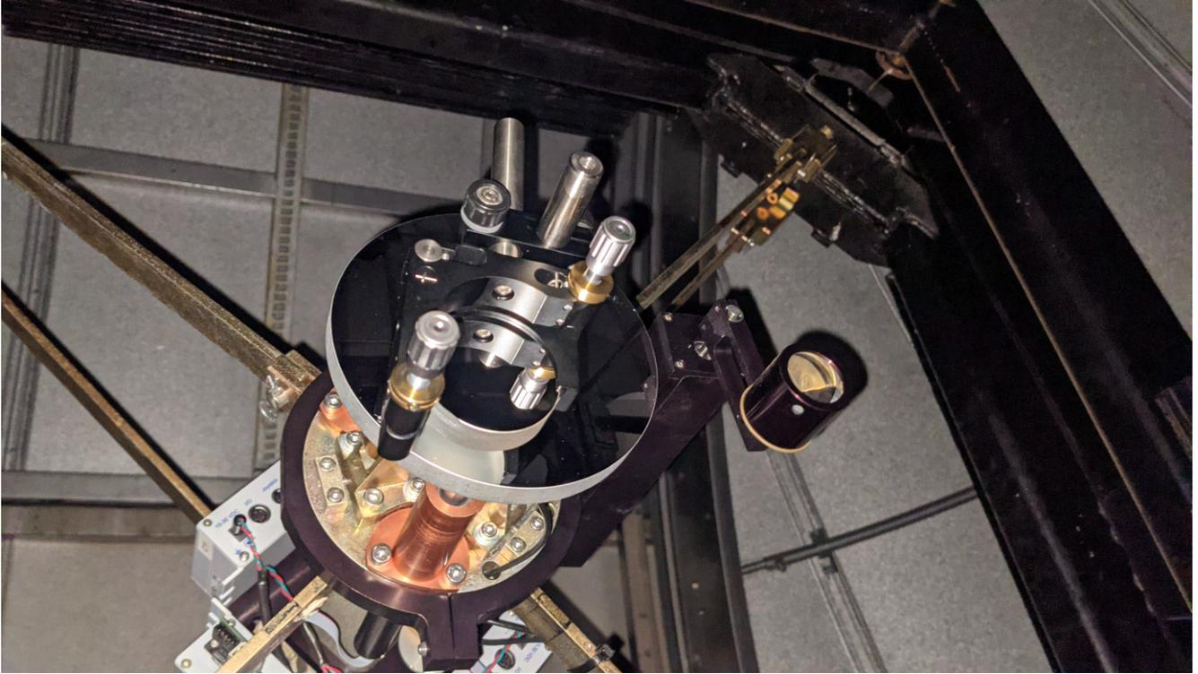
**FIGURE 1.** M2 with the retro mirror mounted.
