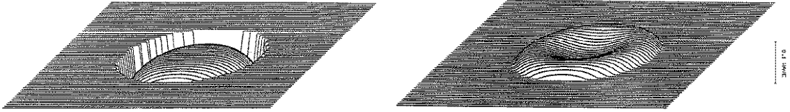
FIGURE 2. The contour plot at left is the wavefront when there is -0.0005 conic constant error on the primary mirror. The p - v is 0.094\lambda . The plot at right shows that the wavefront p - v is reduced to 0.025\lambda by moving 0.003 mm away from the primary mirror.
