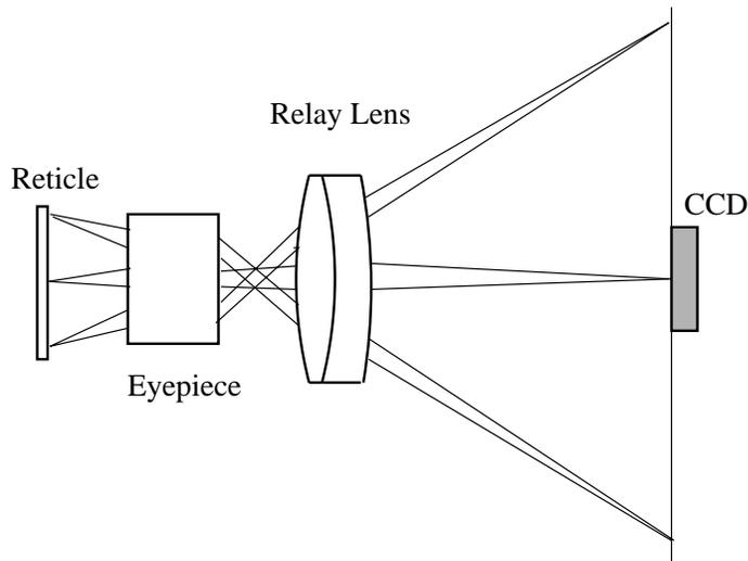
**FIGURE 1.** Reimaging the telescope image and the reticle onto a CCD by a relay lens.
